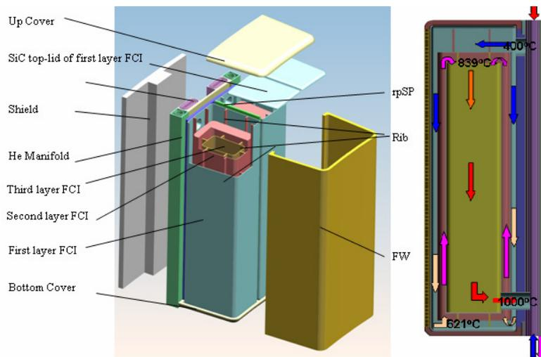
Fig. 4 FDS-III HTL blanket module structure (left) and LiPb flow scheme inside module (right)
