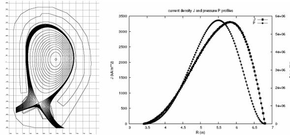
Fig. 1: The magnetic configuration and the profiles of current density and plasma pressure in FDS-III
