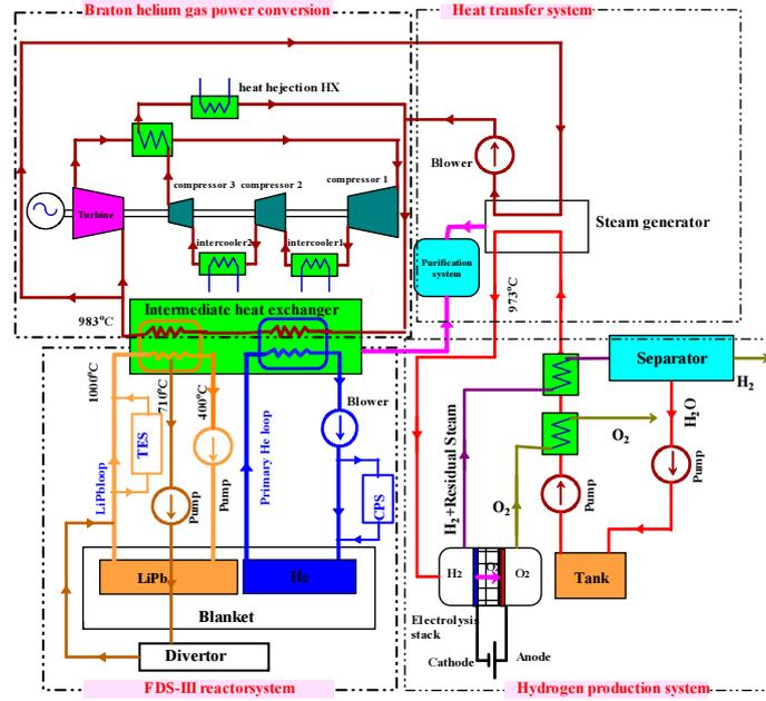
Fig.9 Diagram of FDS III-based hydrogen production
