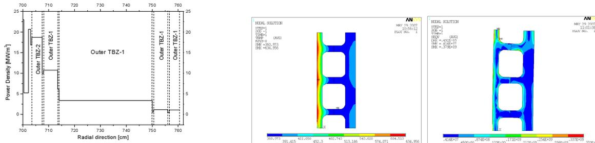
Fig.5 The nuclear heating density Fig.6 Thermal and stress distribution at the First Wall
