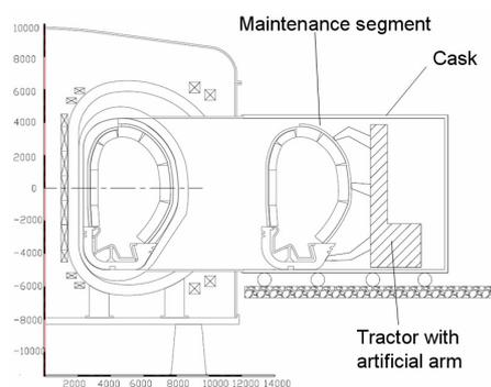
*Fig. 3. Process of one maintenance unit removed by tractor in cask*
